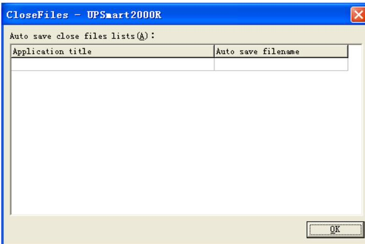
If UPSmart2000R automatically shut down and automatically save documents caused by the utility failure or low battery, when start up the system next time, it will display the above window, which contain the system closed procedure and the file name opened in last time.
