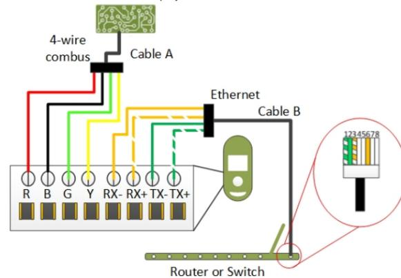
Figure 2 – HD77 Camera - Dual Cable Wiring
