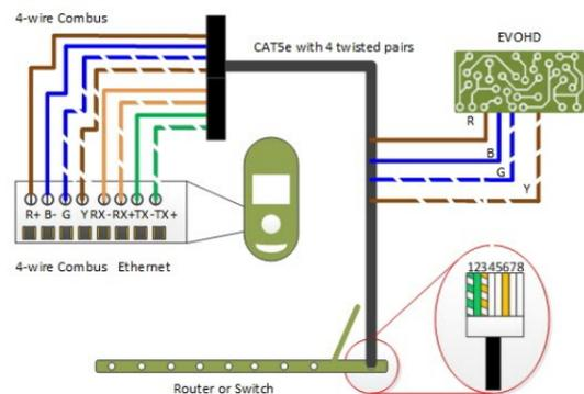
Figure 1 – HD77 Camera - CAT5e Cable Wiring
