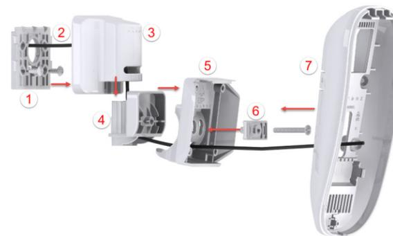
Figure 4 – Mounting HD77 Camera with Swivel Brackets
