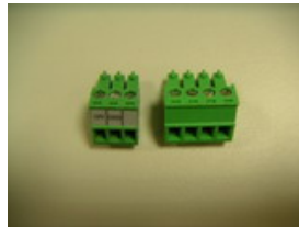
Terminal Blocks for Power & DI/O
